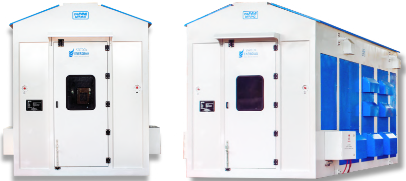
2x558kW Rectifiers Containerised - 3600A/ 155V for NTPC, Leh Green Hydrogen Mobility Pilot Project (Forced Air-Cooled; Outdoor Container Type)
