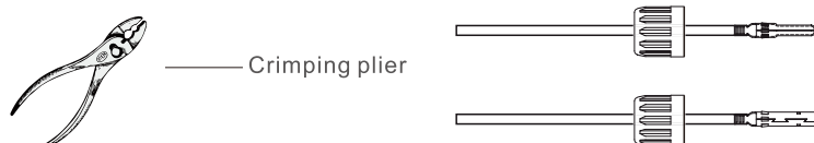
Figure-5.4 Crimp the pin to the wire
