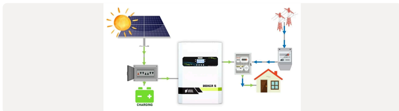
Block diagram of installation. Boxer connects solar panels, battery, grid and home loads.
