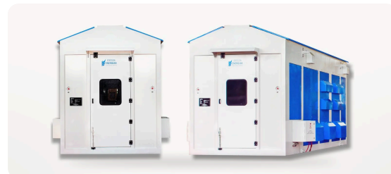
Two 558 kW containerised rectifiers, 3600 A / 155 V, forced air-cooled, for a green hydrogen mobility pilot.
